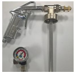
Once cleaned, replace the outer nozzle and re-attach the cleaning container. Then spray through fresh cleaning solvents to make sure the tube and internal body are completely clean. Your gun is now ready to store.
