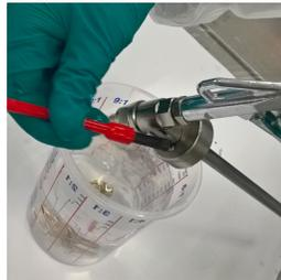
Detach the gun from the air supply, unscrew the outer nozzle and submerge in thinners and clean with a short hair brush.
