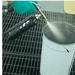
Attach a bottle filled with cleaning solvents to the gun and pull and hold the trigger for 10-15 seconds. This will clean the inside of the pick-up tube.
