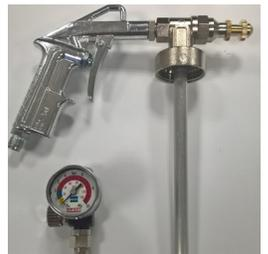
Once cleaned, replace the outer nozzle and re-attach the cleaning container. Then spray through fresh cleaning solvents to make sure the tube and internal body are completely clean. You are now ready to paint again.
