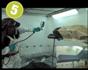
**EPOXY PRIMER APPLICATION**Use an HVLP Gravity Feed Spray Gun at 30 PSI with a 1.4-1.8mm gun tip. You can also apply with a roller or brush. Apply 2-3 coats allowing 10 minutes flash off between coats. Topcoat with Raptor Protective Coating in as little as 60 minutes or as long at 7 days without the need to resand Raptor Epoxy Primer.
